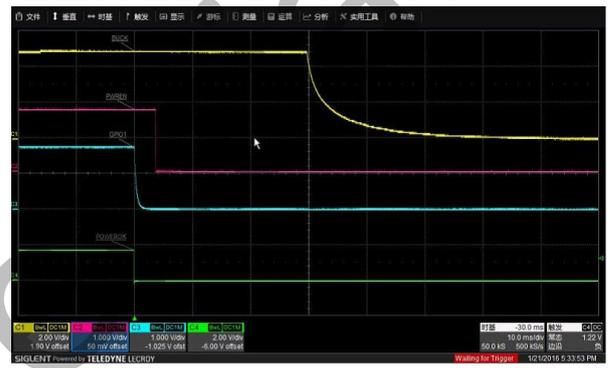
CH1: BUCK, 2V/div; CH2: PWREN, 1V/div; CH3: GPIO1, 1V/div; CH4: POWEROK, 2V/div
