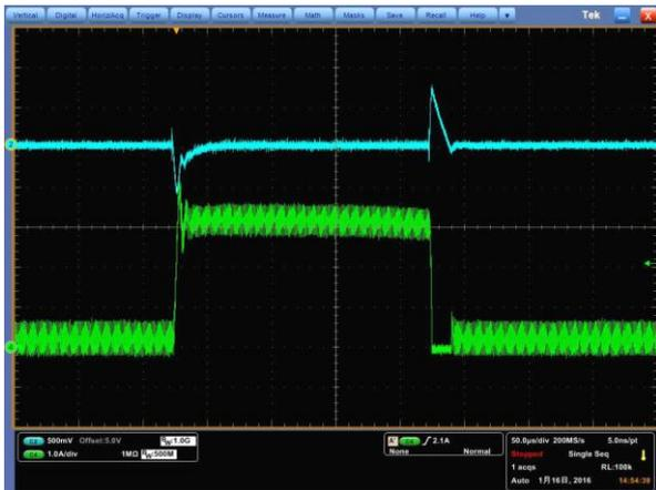
ACIN= 8.4V,  $I_L = 0.4A \sim 4.0A$ ; CH2: Vout, 500mV/div;
