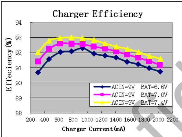
Figure 3. 2 Cells Battery Charger Efficiency vs. Charger Current (ACIN=9V)
