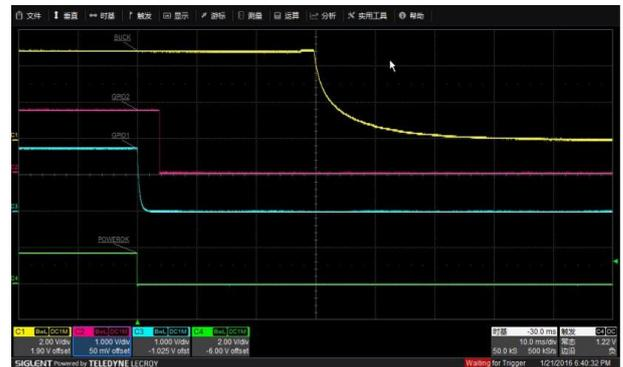
CH1: BUCK, 2V/div; CH2: GPIO2, 1V/div; CH3: GPIO1, 1V/div; CH4: POWEROK, 2V/div
