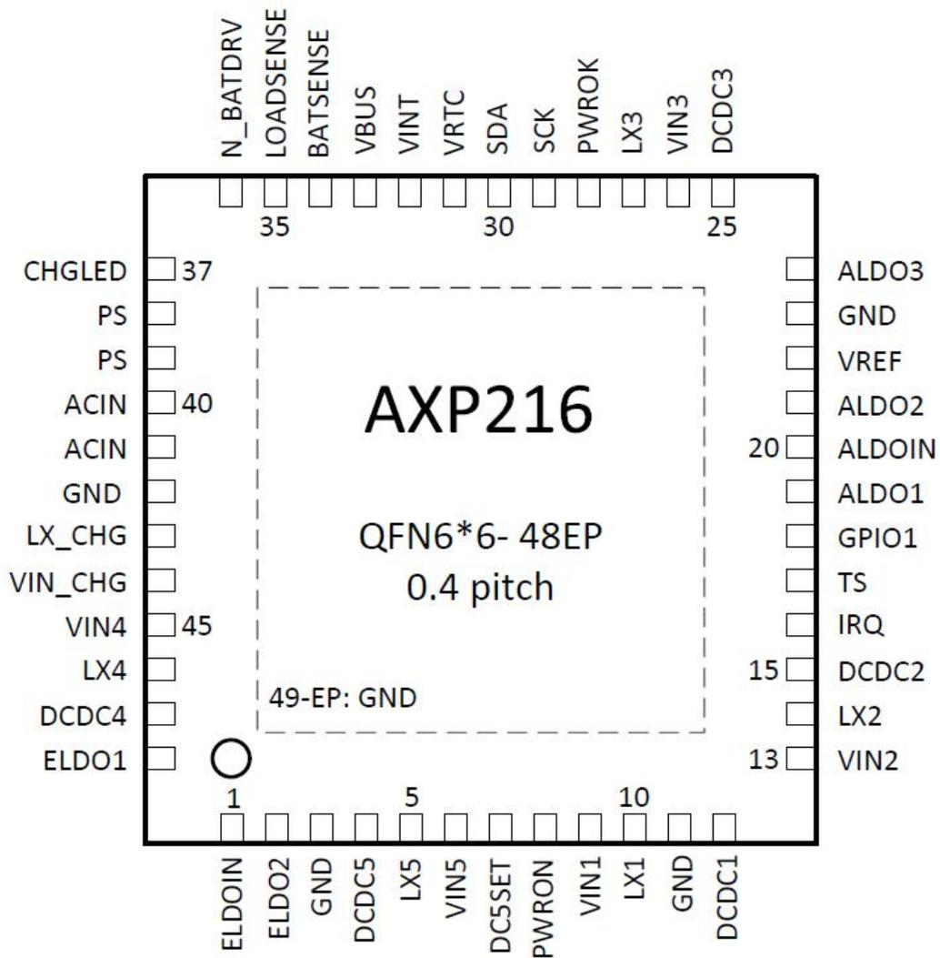
Figure 2. AXP216 Pin Configuration
